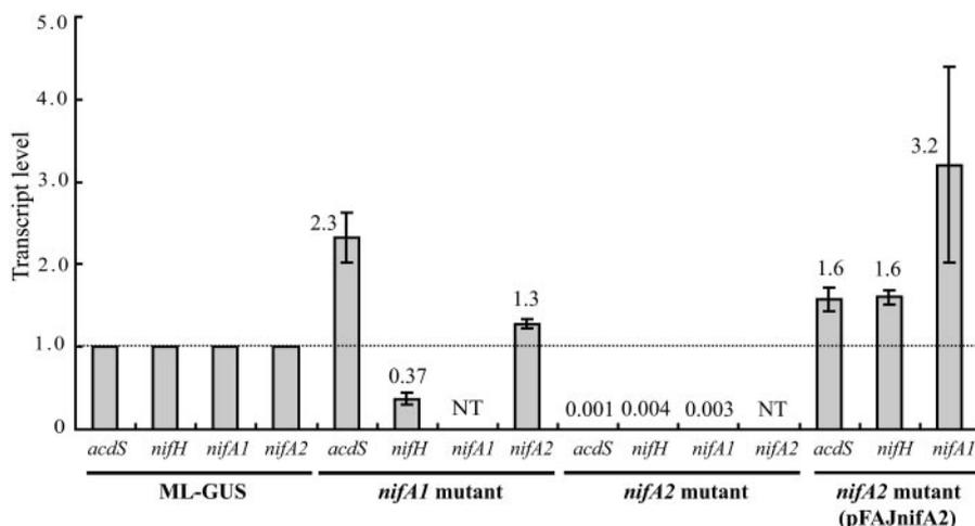
FIG. 4. Quantitative real-time RT-PCR analyses for the *acdS*, *nifH*, *nifA1*, and *nifA2* genes in *M. loti* MAFF303099 for roots at 10 DAI. The relative transcript level for each target gene was normalized to the *gusA* copy number, and the transcript levels for ML-GUS were defined as 1.0. The values are means of three independent experiments, and the error bars indicate standard errors. NT, not tested.
